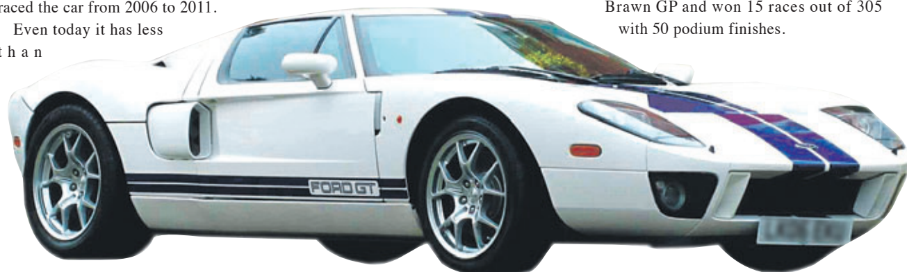
FORD GT: Boasts a hand-crafted 550bhp V8 engine and six-speed manual transmission.
