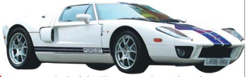
FORD GT: Boasts a hand-crafted 550bhp V8 engine and six-speed manual transmission.
