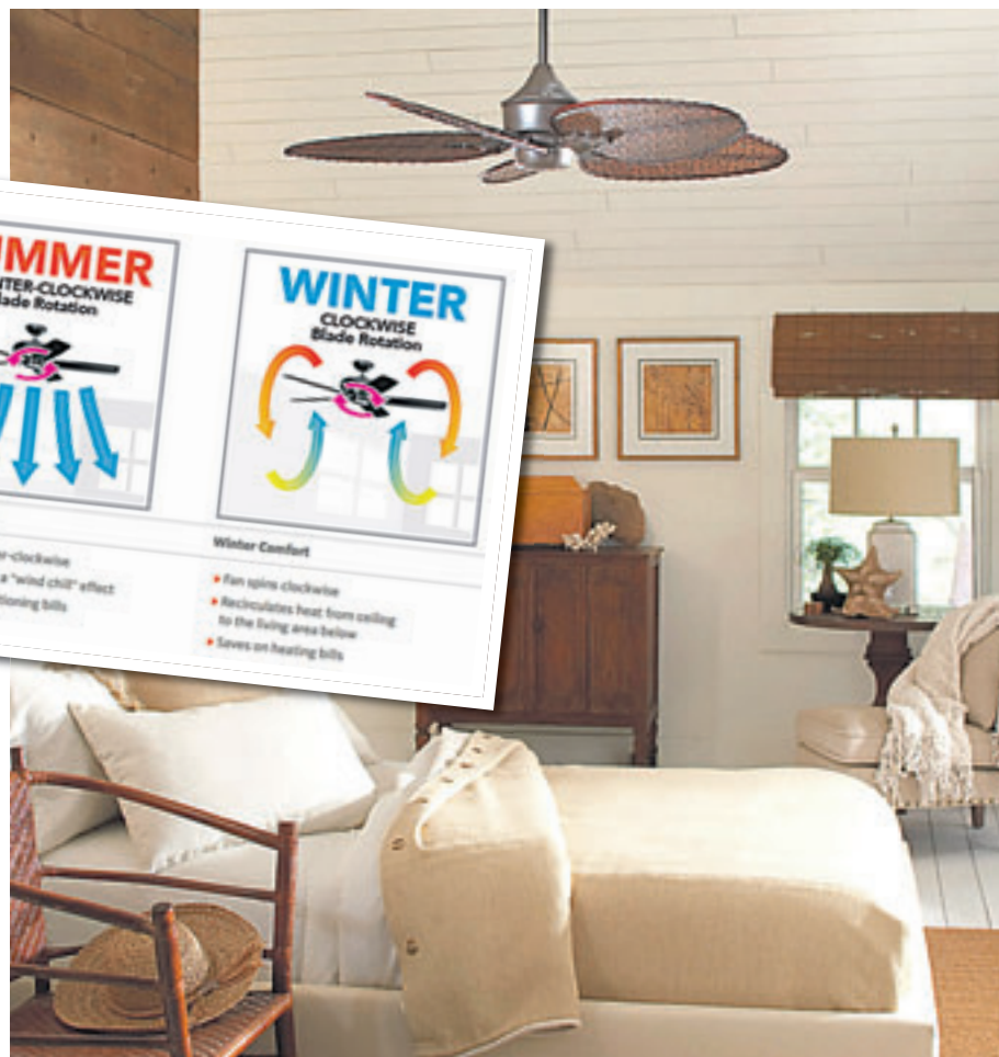
WINTER TIME: Spinning clockwise the fan will draw the room air upwards.
